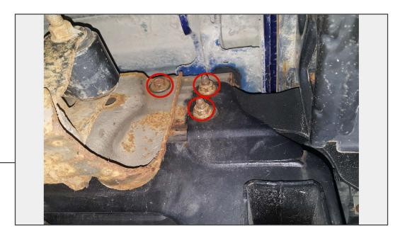
Remove the (2) 18mm nuts, double bolt plate, and 15mm bolt that holds the bumper to the top frame rail. Remove bumper from vehicle.
