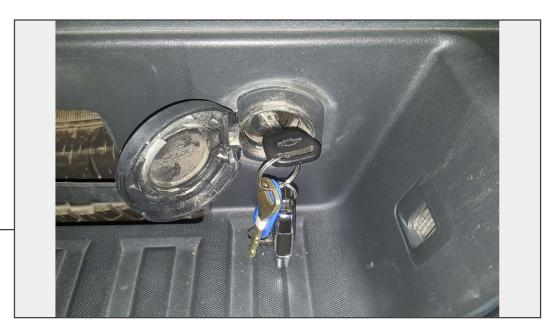
Using your factory ignition key, turn the spare tire lock clockwise and remove the spare tire lock from the factory bumper.
