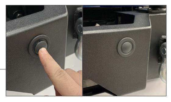
No Sensor: Press the plastic cap into the backup sensor housing through the face of the bumper.
