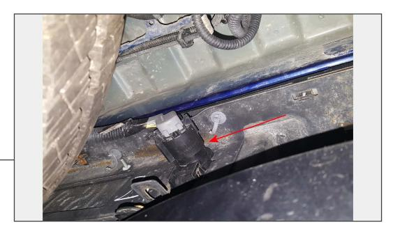
Unplug the factory license plate light harness and the trailer plug connector.
