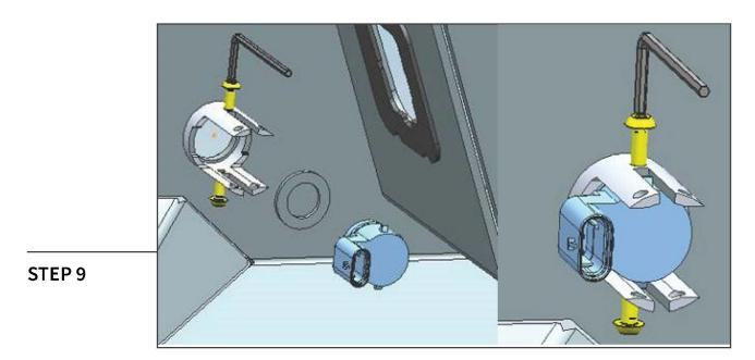
**Optional Sensor Mounting:** Using the provided M4 Allen screws lightly tighten the screws into the sensor to hold it in place.
