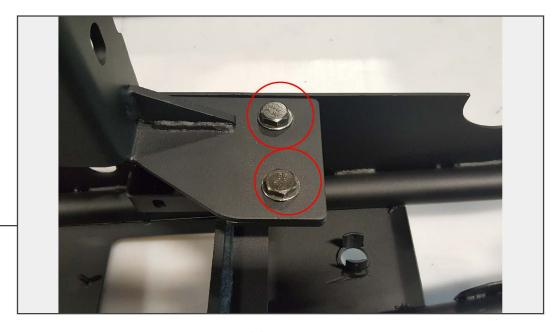
Attach the new bumper to the bumper bracket using (2) M12x1.75x35mm bolts, flat washers, and lock nuts. Do not fully tighten.
