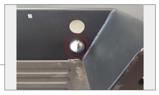
Insert the included license plate light in the new bumper. The aftermarket light only requires a 12V power source, it is grounded through the bumper. Use a test light to determine which factory wire is the 12V+ for the factory light. Splice the aftermarket power supply into the corresponding factory wiring.
