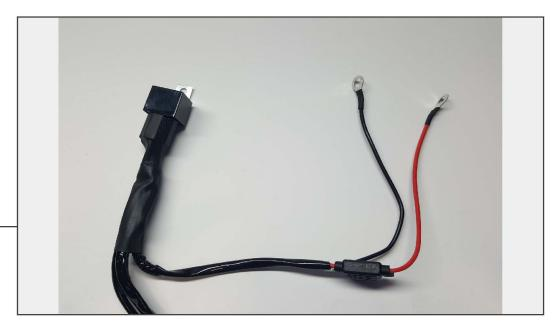
Optional LED light wiring: Install the Red 12+ volt wire to the positive battery terminal. Connect the black ground wire to the negative battery terminal. Secure any additional wiring away from hot/moving drivetrain components.
