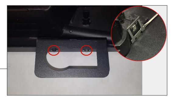
Install the trailer plug bracket that fits your vehicle by using the (2) M6x1.0x15mm bolts, washers, and lock nuts. Reinstall the trailer plug into the new bracket. If it does not clip in, use a small screw driver to expand the clips.
