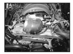
Step 15 Install the 90° boot on throttle body with the short side on the throttle body and clamp on the throttle body side to secure the boot in place. Install a second clamp but do not tighten at this time.
