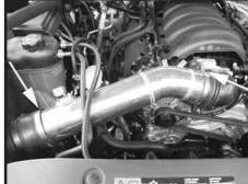
Step 16 Install the intake tube as shown and once in position tighten clamps.
