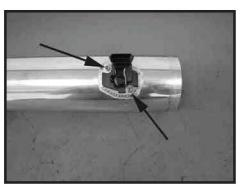
Step 8 Insert and fasten the MAFS onto the intake tube with the provided machine screws.
