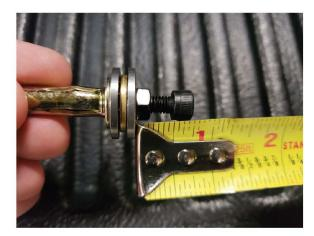
Step 3\\ Assemble the nutsert tool as follows: nutsert, washer, bearing, washer, nut, Allen bolt. Adjust the tool so that there is 3/4" between the flat washer and the head of the Allen bolt.
