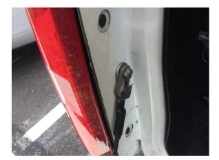
Step 1\\ Remove the lift gate strap and loosen the 13mm lift gate bolt.
