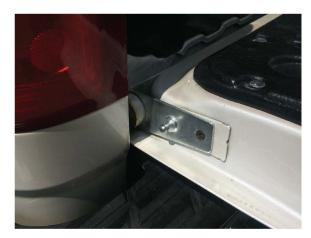
Step 5\\ Apply blue thread lock to the threads of the (1) M6 x 1.0 x 20mm bolt, and secure the lower ball mount plate to the tailgate. Torque the bolt to 8ft-lbs.
