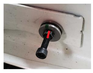
Step 4\\ Place the nutsert assembly in the tail gate, if it is a tight fit gently tap the assembly in with a rubber mallet. Mark the nut for a visual reference when turning. Hold the Allen head bolt steady and turn the nut (9) full rotations. \*\*Note: Do not turn the Allen bolt. Over-tightening the nutsert will damage it.
