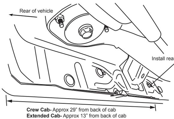
**Note: U-nut may be needed if threaded insert is not present on vehicle**
