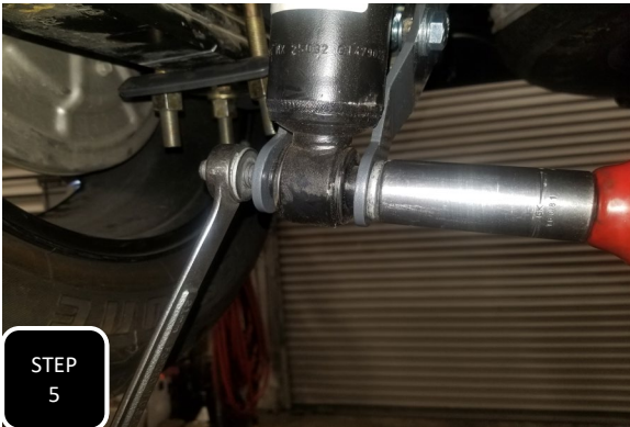
Step 5 Attach the shock to the extender using the factory hardware and tighten.
