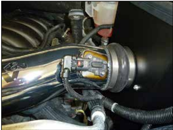
25. Connect the mass air sensor electrical connection.
