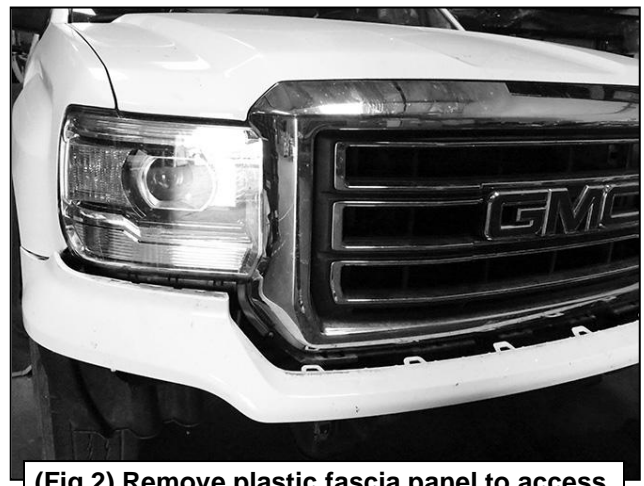
(Fig 2) Remove plastic fascia panel to access hardware attaching bumper to top of bracket
