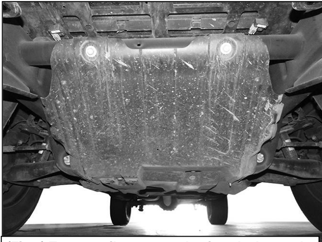
(Fig 1) Temporarily remove plastic splash guard.
