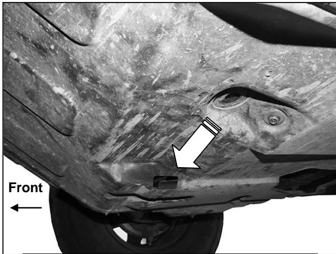
(Fig 4) Reinstall splash guard. Note insert flat passenger side of Bracket through slot and between skid plate and crossmember
