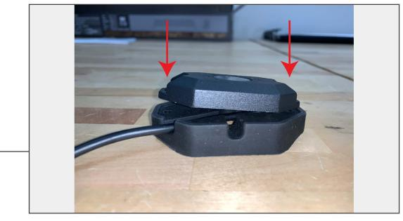
Install the Rock Lights to the appropriate mount and vehicle location using (2) Allen bolts, (2) flat washers, and (2) nuts.
