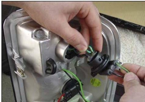
Plug the pigtails into the stock wire harness.
