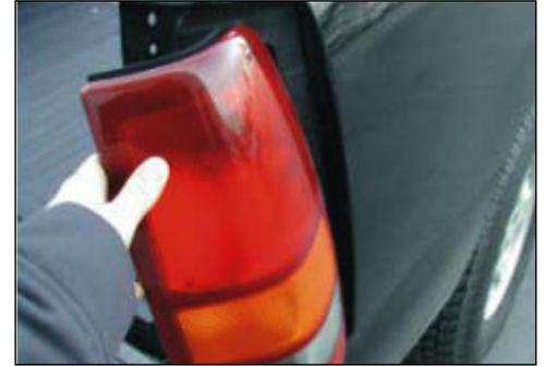
Once the screws are removed, you will be able to pull tail lens straight out.
