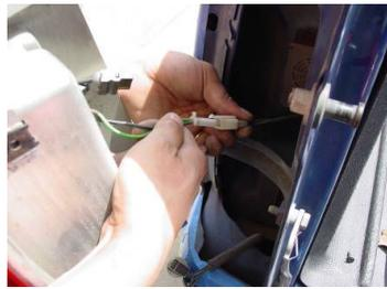
Step 8: Connect the resistor
