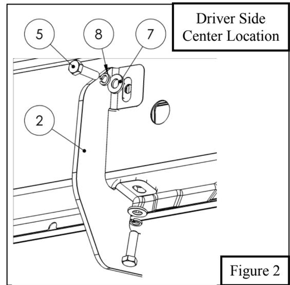
5. Locate (1) Center Mount Bracket (Item 2-3). Loosely secure Center Mount Bracket to the rocker panel using (2) M8 hex head bolt (2) M8 flat washer, and (2) M8 lock washer. See **Figure 2**. Refer to **Page 3** bracket orientation figures.
