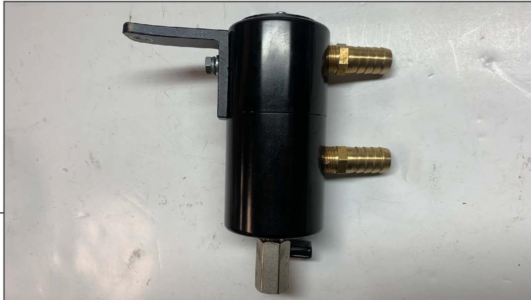
Install the supplied bracket to the oil separator using (1) M6x1.00 14mm bolt, (1) M6 lock washer, (1) M6 flat washer. Install the ball valve on the bottom of the oil separator, use thread sealant to ensure a leak free installation.
