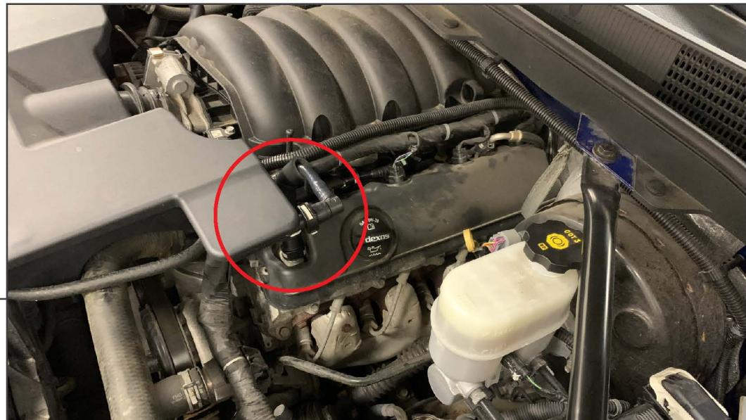
Locate the PCV line connecting the valve cover to the intake . Depress the gray locking tab and pull to connector away from the vehicle.
