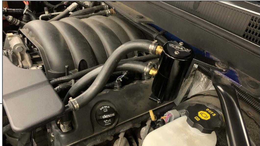
Route the supplied vacuum lines connecting the bottom port of the oil separator to the port on the valve cover. Connect the top of the oil separator to the intake manifold port. Secure the lines with the supplier hose clamps. Installation is now complete. Empty oil separator as needed.
