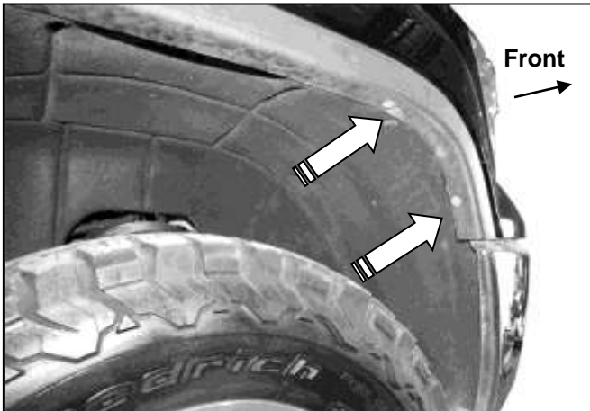
(Fig 1) Locate and remove screws attaching ends of fascia body panel to front fenders
