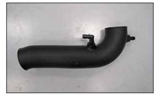
6. Install the provided 90° and straight vent fittings into the K&N $^{\! \tiny @}$  intake tube as shown.
