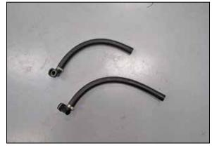
9. Install the provided quick disconnect fittings into one end of each hose and secure with the provided hose clamps
