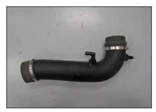
7. Install the provided coupler hoses onto the K&N® intake tube and secure with the provided hose
