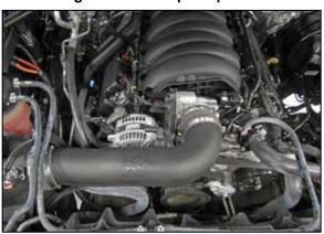
8. Install the intake tube assembly onto the air filter housing and then onto the throttle body, adjust the tube for best fit and then secure with the provided hose clamps.
