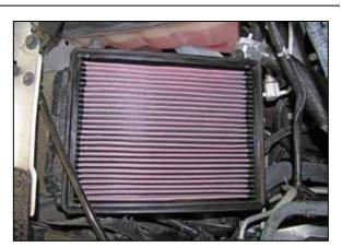
5. Install the K&N $^{\circ}$  air filter into the lower filter housing and then reinstall the upper housing and secure with the factory hardware.
