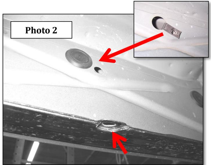
**Step-2** Attach one of the driver side brackets to the rocker panel using the U-Nut, (1) M8 hex bolt, (1) 5/16" lock washer and (1) 5/16" flat washer, and to the pinch mold using (1) M8 hex bolt, (2) 5/16" flat washers, (1) 5/16" lock washer, and (1) M8 hex nut. Leave the nut and bolts loose for final adjustment, (**Photo 3**).
