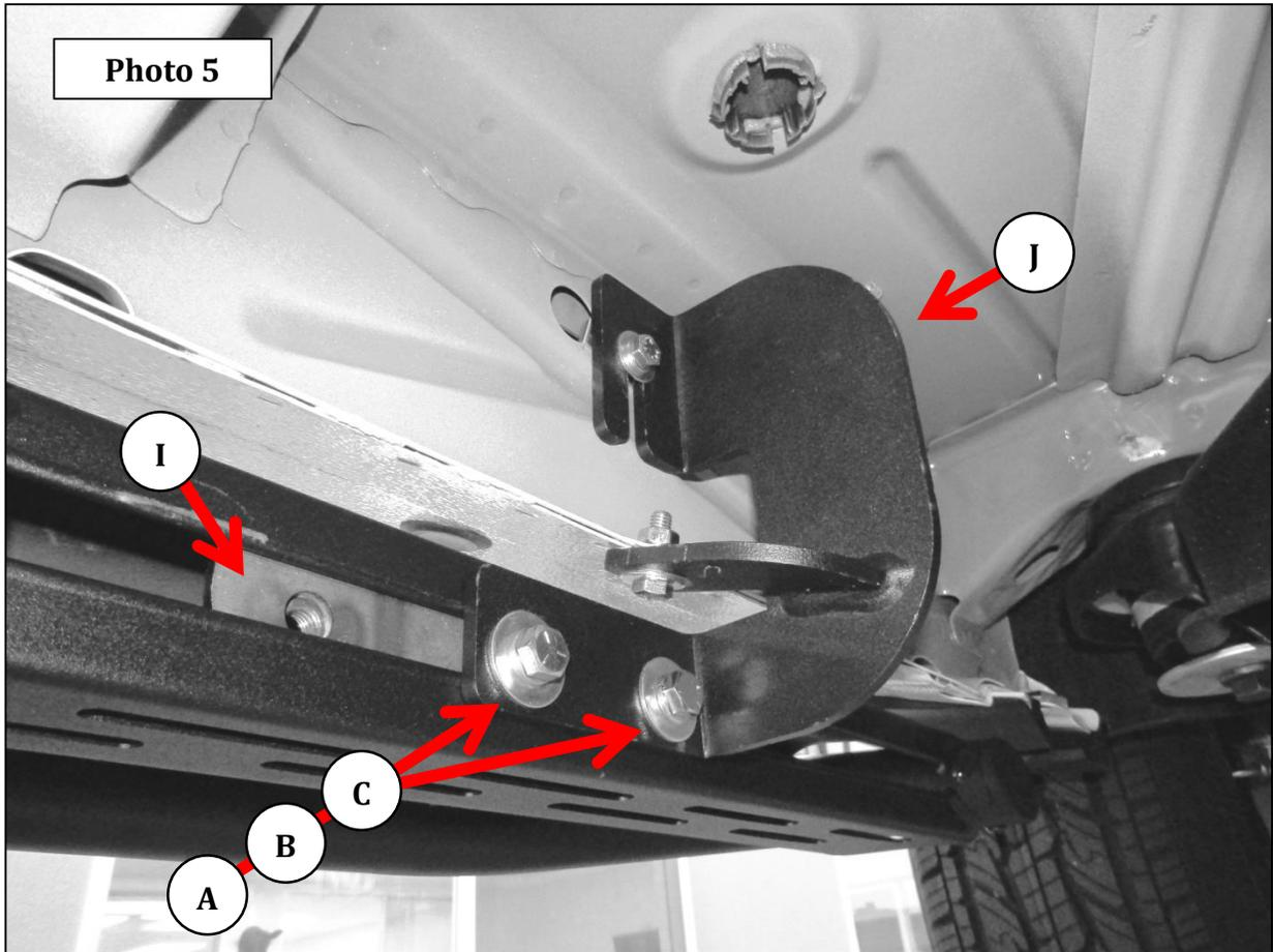
**Step-5** Align the Dominator D1 side step with the vehicle and tighten all bracket and side step nuts and bolts. Repeat the above steps to install the passenger side brackets and Dominator D1 side step.
