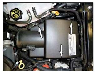
7. Loosen the three screws that secure the air filter lid onto the air filter base. Remove the lid and hose assemble and factory air filter from the vehicle.
