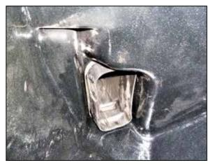
17. Engage the fresh air duct into the K&N air filter housing and then secure it with the factory retaining clip.
