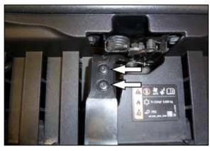
2. Remove the two screws that secure the hood release lever and then remove the lever from the vehicle.
