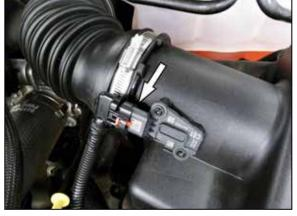
6. Disconnect the mass air sensor electrical connection.
