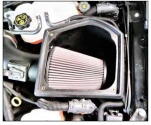
26. Install the K&N air filter into the air filter housing and onto the filter adapter, then secure with the provided hose clamp.
