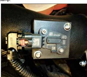
25. Reconnect the mass air sensor electrical connection.
