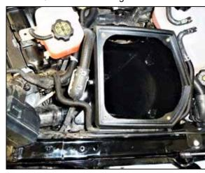
16. Install the K&N air filter housing into the vehicle so the mounting grommets insert into the factory mounting holes and then secure with the factory mounting nut.
