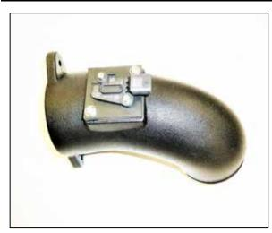
22. Install the mass air sensor into the K&N intake tube and secure with the provided hardware. Note the direction of the mass air sensor when installed should be as in the photo.
