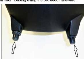
15. Remove the two-air box mounting grommets from the factory air filter housing and install them onto the K&N air filter housing as shown.
