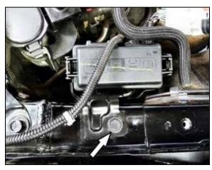
12. Remove the relay box mounting bolt shown.
