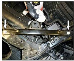
10. Remove the two bolts that secure the strut brace and then remove the strut brace from the vehicle.
