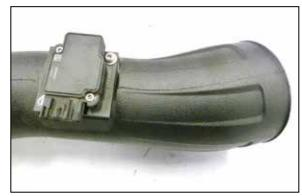
16. Install the MAF sensor assembly into the K&N intake tube and secure with the provided hardware like image shown above.
