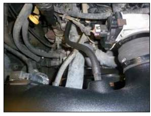
19. Connect the provided 3/8" crank case hose to the engine fitting and fitting on intake tube.
