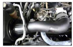
17. Now install the intake tube assembly and position to the air box and throttle body. Tighten clamps using 5/16" socket or nut driver. Note: Do not over tighten clamps.
