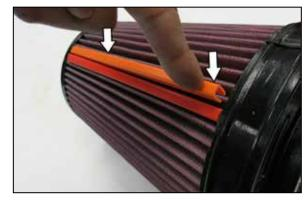
12. Attach the filter clips to the pleats on the air filter align and push down. Passenger side filters, place orange clip on top and red on bottom.
