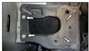
10. Remove the OEM air box bracket, and save 3 bolts for the K&N air box install.
