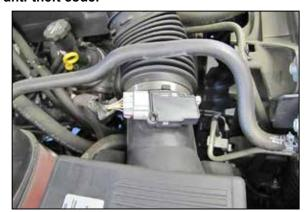
2. Disconnect the mass air electrical connection.
