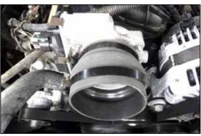
14. Install the hump hose with clamps to the throttle body. Do not tighten.
