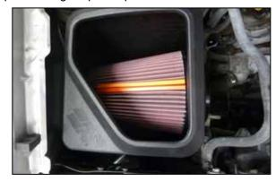
13. Install the air fiter into the K&N air box.
