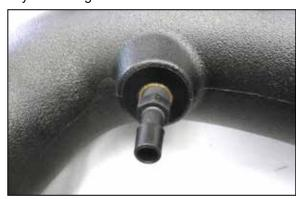
15. Install the provided  $\frac{1}{4}$ " NPT fitting into the K&N intake tube as shown.
