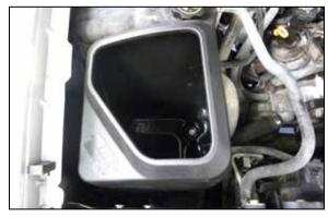
11. install the K&N air box and secure using the 3 bolts from previous step.
