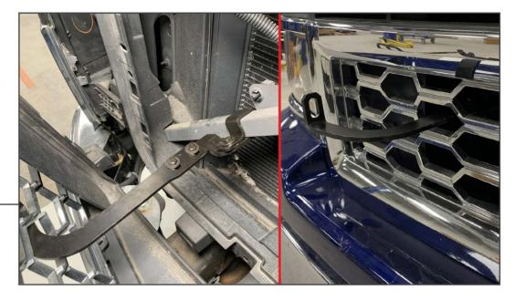
While holding the vehicle grille, insert the upper mounting brackets through the holes in the grille. The upper mounting brackets must be in line with the lower mounting brackets. Once aligned, tighten the 'U' Brackets and the upper mounting brackets to the M6 nut plates.
