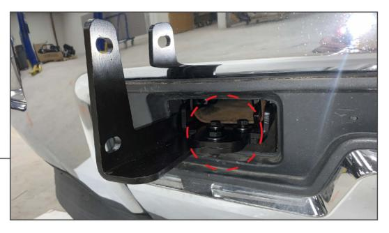
With each frame rail adapter installed, re-install the vehicle bumper using the original hardware. Secure the lower mounting bracket to the frame rail adapter using (3) M8 x 25mm bolts, (3) M8 lock washers, and (3) M8 flat washers.
