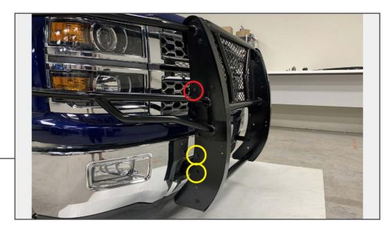
With assistance, lift the assembled grille guard to the vehicle mounting brackets, and secure the bottom of the grille guard using (2) M10 x 30mm bolts, (4) M10 flat washers, (4) M10 lock washers, and (2) M10 nuts per side. Secure the top of the grille guard to the upper brackets using (1) M8 x 30mm bolt, (2) M8 flat washers, (1) M8 lock washer, and (1) M8 nut per side.
