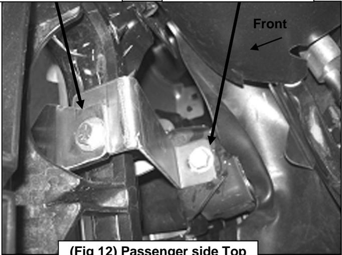
(Fig 12) Passenger side Top Support Bracket pictured
