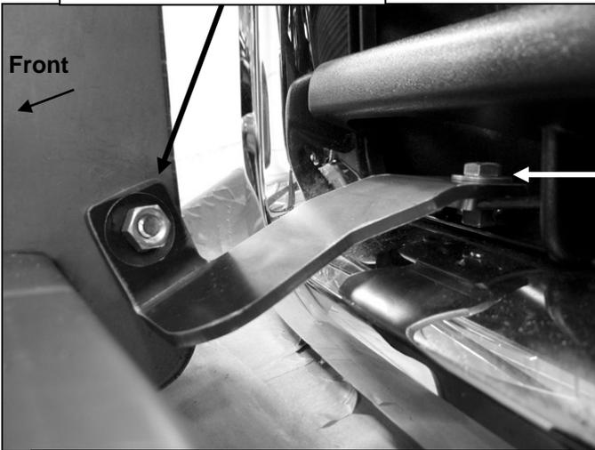
(Fig 15) Passenger side Top Bracket pictured
