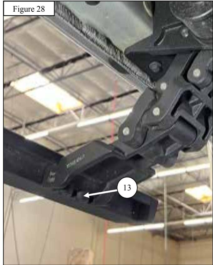
22. Locate and connect the previously routed male connectors from the main wiring harness to the female connectors on each motor linkage assembly. As mentioned previously, the male connector labeled “Front Left” will be connected to the female connector on the front driver side motor linkage, and the “Front Right” male connector should be connected to the female connector on the front passenger side motor linkage. See **Figures 30 & 31** for reference.
