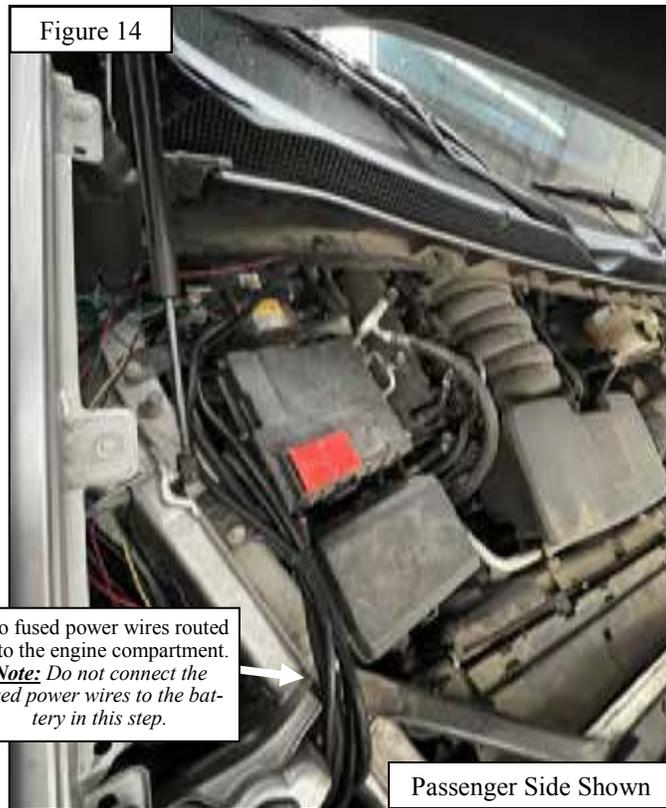
Two fused power wires routed up to the engine compartment.
