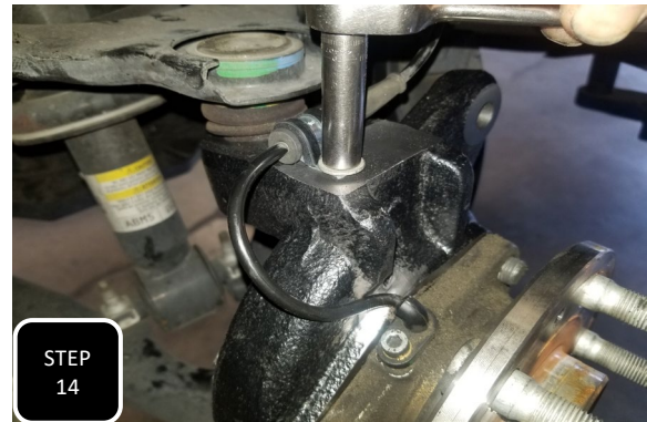
Step 14 Re-attach the ABS sensor using the factory allen head bolt and tighten. Next, attach the ABS wire to the top of the spindle using the provided loom clamp around the rubber grommet on the ABS line and the factory 6mm bolt.
