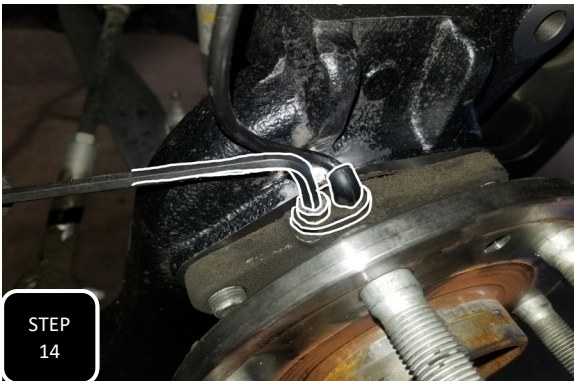
Step 14 Re-attach the ABS sensor using the factory allen head bolt and tighten. Next, attach the ABS wire to the top of the spindle using the provided loom clamp around the rubber grommet on the ABS line and the factory 6mm bolt.
