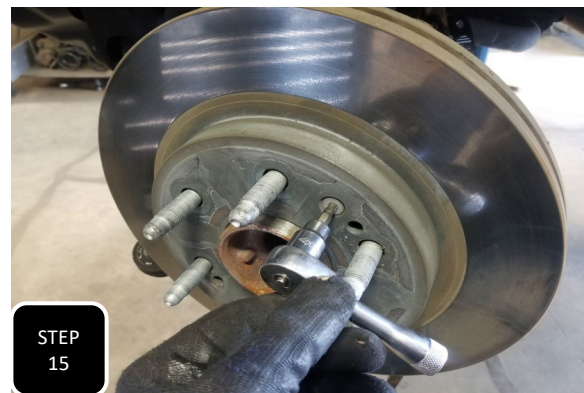
Step 15 Slide the rotor over the wheel studs and secure it using the factory retainer bolt.
