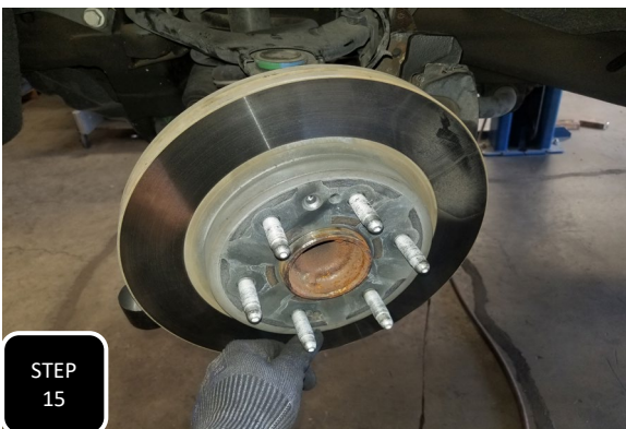
Step 15 Slide the rotor over the wheel studs and secure it using the factory retainer bolt.
