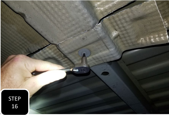
Step 16 Once all the way cut out, remove the mounting bolt in the cut area and remove the cut section of heat shield.
