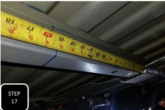
Step 17 Measure and mark a line 15 inches out from the heat shield that you just cut out then draw a cut line up both sides and along the top .
