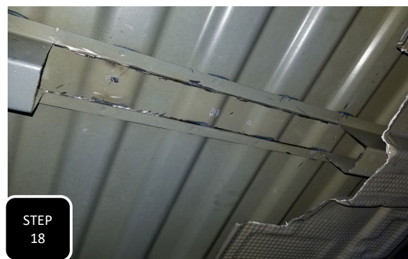
Step 18 Using a suitable cutting device such as a cut off wheel, completely cut out and remove this section of bed rib above the rear differential.
