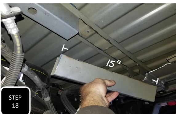
Step 18 Using a suitable cutting device such as a cut off wheel, completely cut out and remove this section of bed rib above the rear differential.
