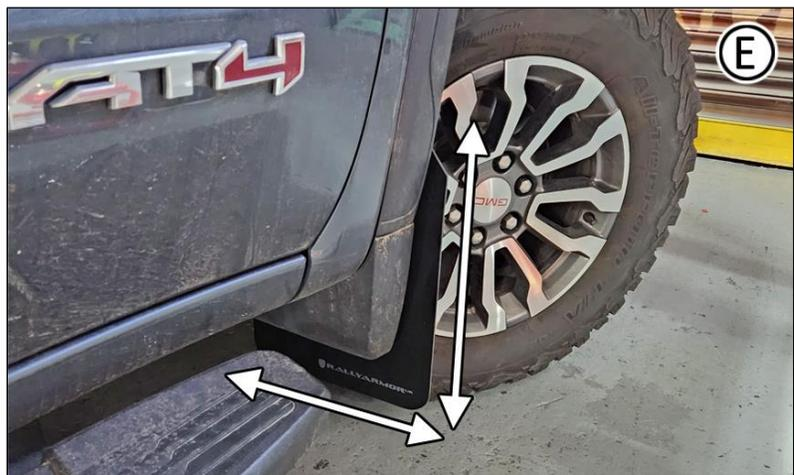
**REAR FLAP** Do not fully tighten fasteners until flap is fully aligned to vehicle.
