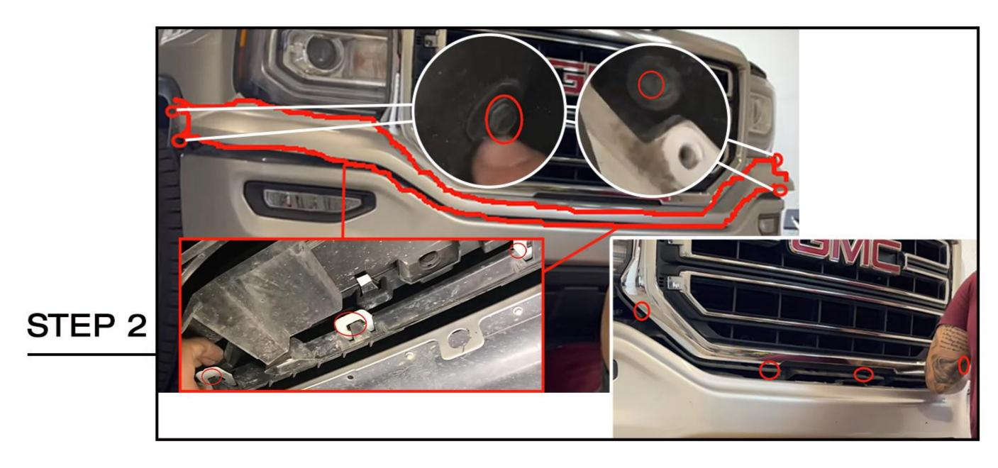
Remove the seven millimeter screw on either side, pop the fender back, there will another seven millimeter screw and remove it. Then push these plastic piece apart underneath the car to remove the circled part. Remove 4 bolts to take the grille off.
