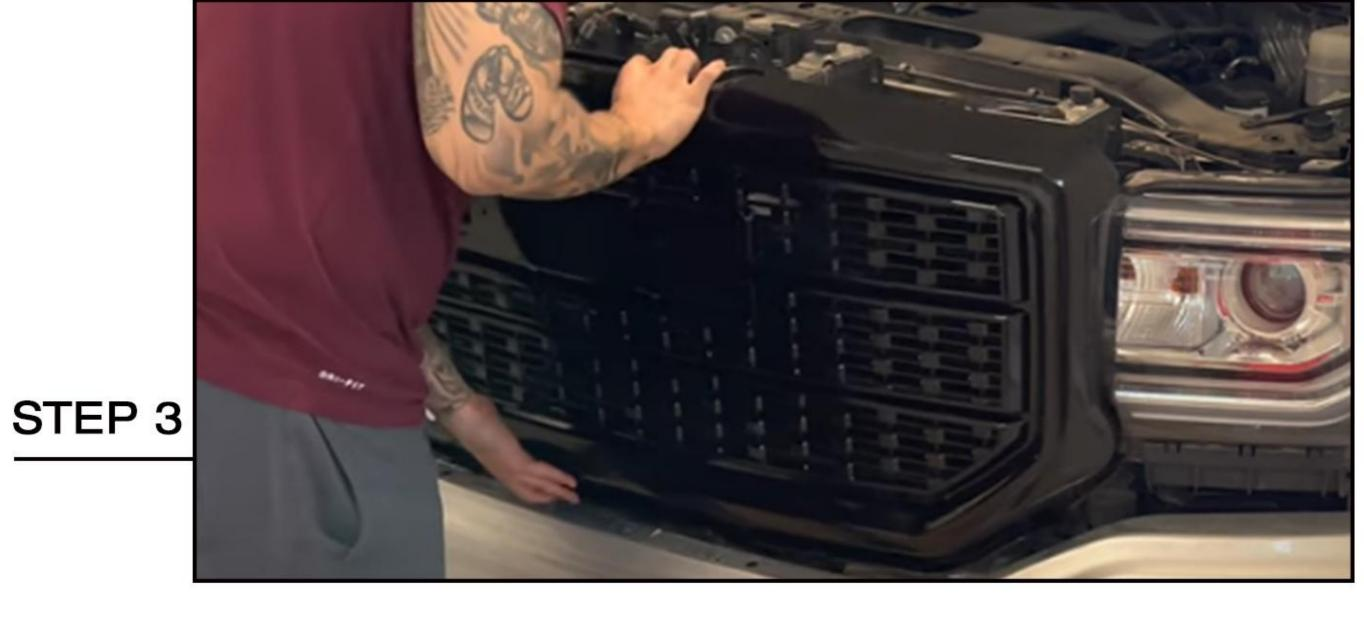
Take out the new grille, remove the emblem from the original grille and install it on the new grille. Then align the new grille to the car and press hard.
