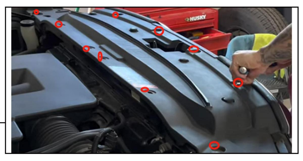
Open the hood, use a trim removal tool to remove 12 push pins to remove radiator cover. Then take four 10-millimeter bolts at the top first.
