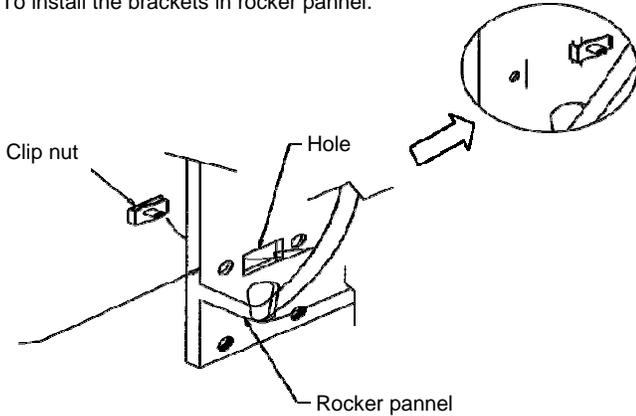
3. Mount bracket and attach with: ( 1 ) 3/8 x 1 1/4" hex head bolt, ( 1 ) 3/8" flat and lock washers, in lower part attach with: ( 1 ) 3/8 x 1 1/4" hex head bolt, ( 2 ) 3/8 flat washer, ( 1 ) 3/8" lock washer, ( 1 ) 3/8" hex nut. **SEE ILLUSTRATION 4.** By each bracket. Leave loose.
