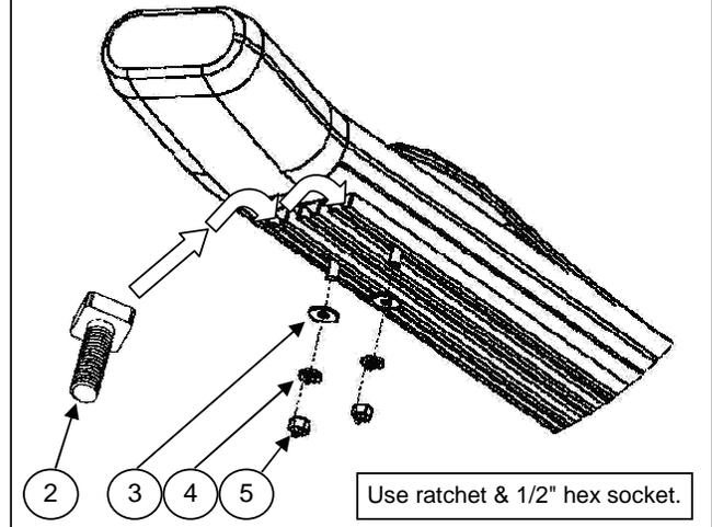
5. If you acquired a Oval side bar widesider 4", place on brackets and attach with: 5/16" square head bolt, 5/16" Flat and lock washer. **SEE ILLUSTRATION 6.** Repeat for the opposite side. Leave loose.
