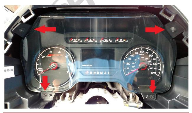
10. Slide the I/C out and remove the connector from the back side. Press the tab in the middle above the arrow and remove. Slide Instrument Cluster out.
