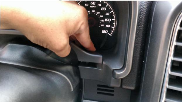
5. Next disconnect the vinyl column cover from the steering column itself. Reach under the backside of the cover and gently pull up, it will disconnect from the steering column rather easily. Completely remove this piece.
