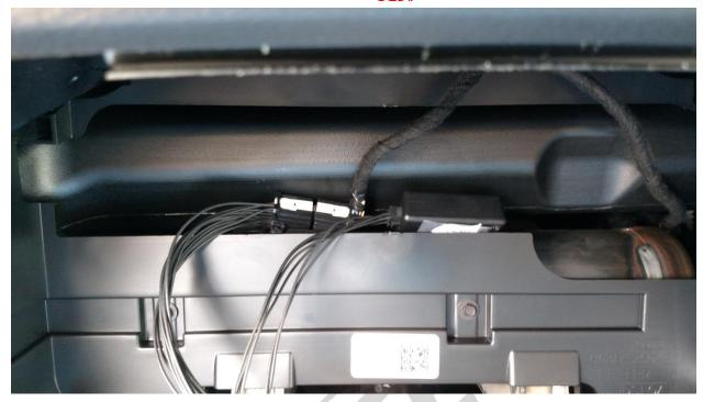
13. Slide I/C back into cavity and insert the Inline Speedometer Module harness into the I/C.
