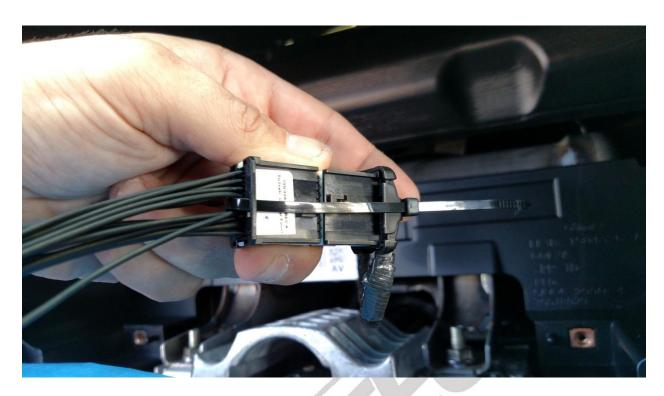
12. For the F150, tuck the harness and module on top of the air duct that runs inside of the I/C cavity to gain clearance for installation. For the F250, access to the top of the duct is limited so insert the harness and module below and orientate them sideways.
