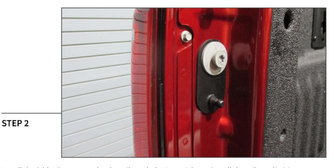
Install the (1) bed mount under the tailgate bolt. Once tight, re-install the tailgate limiting strap.
