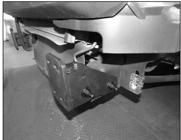
(Fig 6c) Completely installed Driver mounting bracket. Repeat for Passenger side
