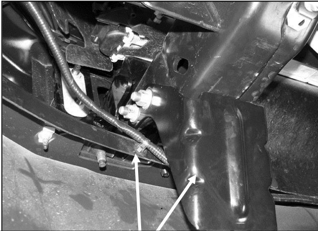
(Fig 1) Driver side lower frame extension and fog light wire harness pictured from behind bumper
