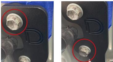
2. Remove the two 12mm bolts securing the hood hinge, while holding the back of the hood. We also highly recommend having someone else hold the front of the hood to make sure it doesn't close when the bolts come out.
