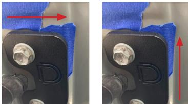
1. Working on one side of the vehicle at a time, mark the location of the hood hinges with tape and tape the edges of the hood to prevent scratching.
