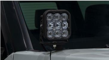
6. Once the brackets are mounted to the hood, refer to the Universal Bracket Info/Mounting Guide, to mount your pods onto the bracket.
