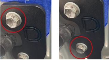
4. Secure the bracket and hood hinge using the factory bolts, ensuring the hood hinge lines up with the tape.
