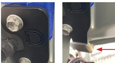
3. Place the ditch light bracket under the hinge and align the holes with the hood hinge. Adjust the bracket to leave a slight gap at the back of the hood before tightening.
