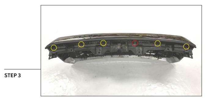
Remove (5) plastic push clips and (1) 10mm bolt to remove the upper grille shroud from the original vehicle grille.
