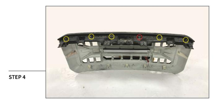
Transfer the upper grille shroud to the new grille reusing the original mounting hardware.
