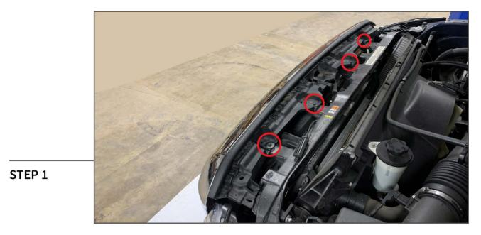
Open the vehicle hood. Locate the (4) 10mm bolts securing the top of the grille to the radiator support. Remove the (4) 10mm bolts.
