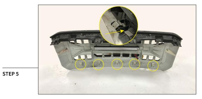
Install the (5) lower retaining clips to the vehicle grille.
