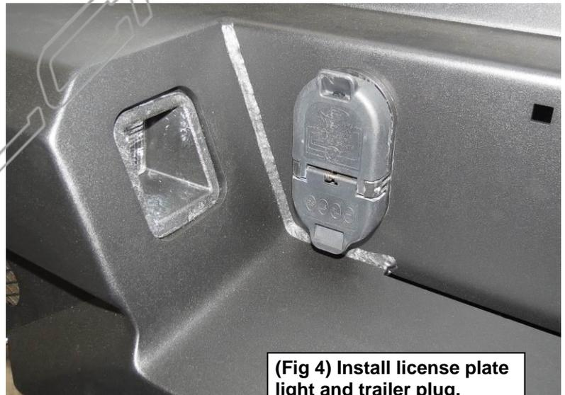
(Fig 4) Install license plate light and trailer plug.
