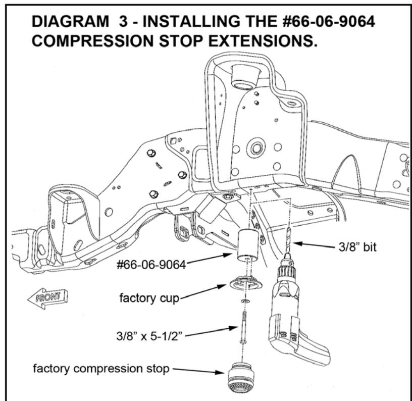
compression stop cup mounting hole in the bottom of the frame to 3/8". Also drill out the hole in the factory cups to 3/8".
