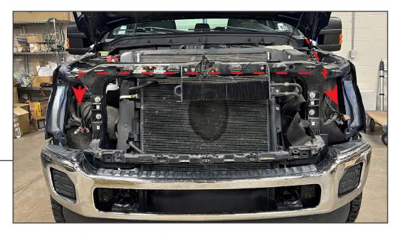
Route the included DRL harness from the vehicle fuse box to each headlight mounting point. Ensure to route the harness away from any hot/moving components.
