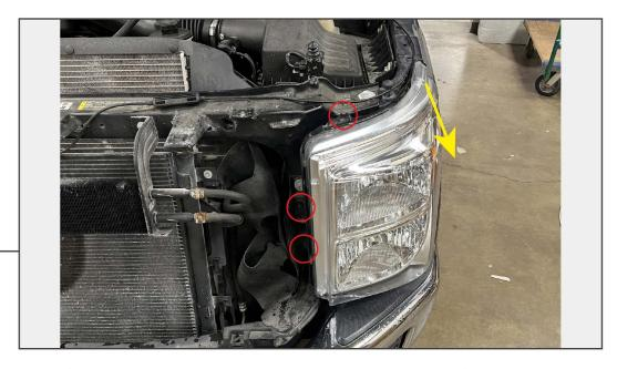
Remove (3) 10mm bolts from the headlight assembly. With the bolts removed, firmly pull the headlight assembly away from the vehicle to dislodge the retaining pin.
