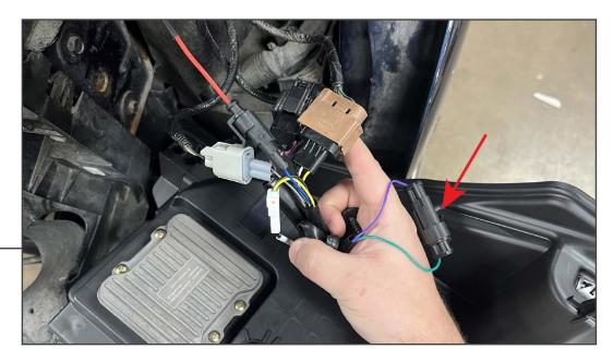
**Turn Signal Sequence On/Off:** Plug in/Unplug the designated connector to toggle turn signal sequence feature.
