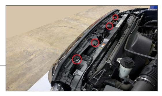
Open the vehicle hood. Locate the (4) 10mm bolts securing the top of the grille to the radiator support. Remove the (4) 10mm bolts.
