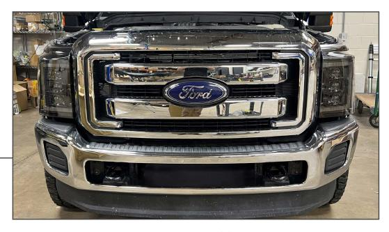
Secure the new headlights into the vehicle reusing the original (3) 10mm bolts. Then, install the grille to the vehicle reusing the original (4) 10mm bolts.
