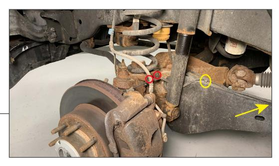
Remove (2) 10mm bolts from the ABS sensor wiring, and release the wiring from the control arm retainers.
