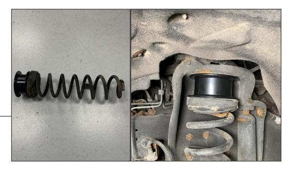
Place (1) coil spring spacer above the coil spring and spring isolator. Install the coil spring assembly into the vehicle. Ensure the bottom of the coil spring fits to the notch.
