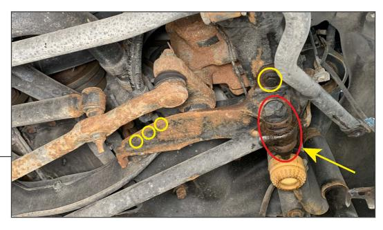
From under the vehicle, loosen and remove the 30mm bolt securing the track bar to the track bar bracket. With the track bar removed, remove (3) 21mm nuts and (2) 18mm bolts to remove the bracket from the vehicle.
