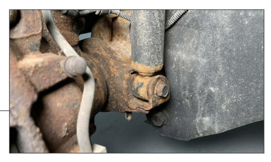
Remove (1) 18mm bolt from the bottom of the shock absorber.
