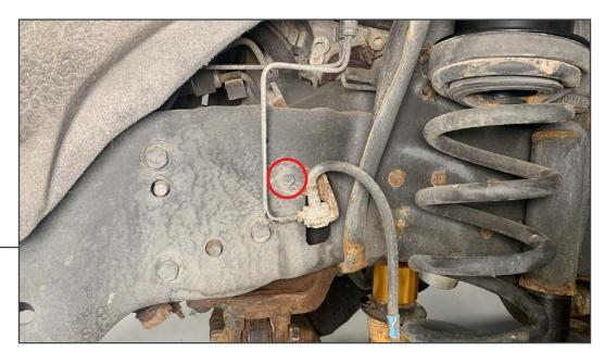
Remove (1) 13mm bolt securing the brake line to the frame.
