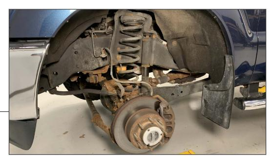
Lift and support the vehicle frame using a floor jack and jack stands. Once supported, remove the wheels from the vehicle. Once supported, place a floor jack under the vehicle axle with minimal pressure on the axle.
