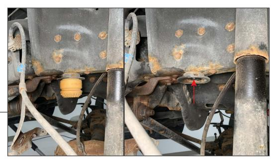
Firmly pull down on the yellow bump stop to remove it from the carrier. Remove the bump stop carrier from the frame by removing (1) 10mm bolt.
