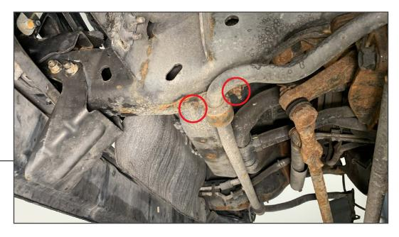
Remove (2) 15mm nuts from the sway bar mount, and allow the sway bar to lower.
