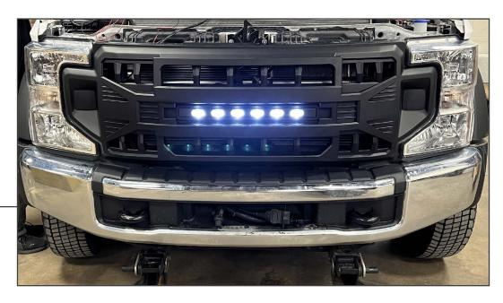
Press the grille to the vehicle to engage the lower clips. Then, follow steps1-4 in reverse order to re-install the grille to the vehicle using the original hardware.
