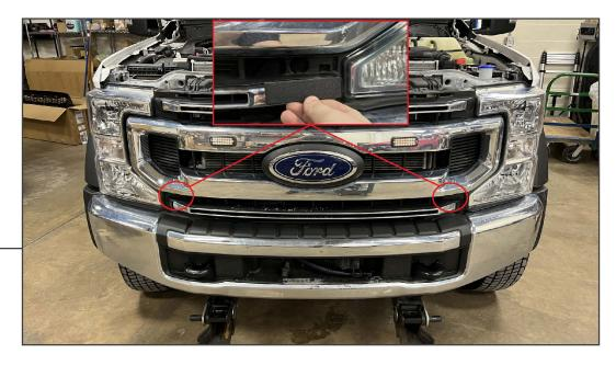
Along the bottom of the grille, locate the bolt cover panels. Using a small pry tool, pry the panel to slide the cover towards the center of the grille. Then, lift the panel away from the grille.
