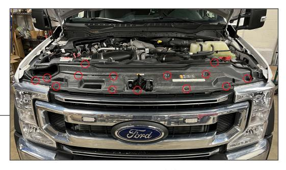
Open the vehicle hood. Remove the radiator cover by removing (14) plastic push clips. With all clips removed, lift the radiator cover away from the vehicle and set aside.
