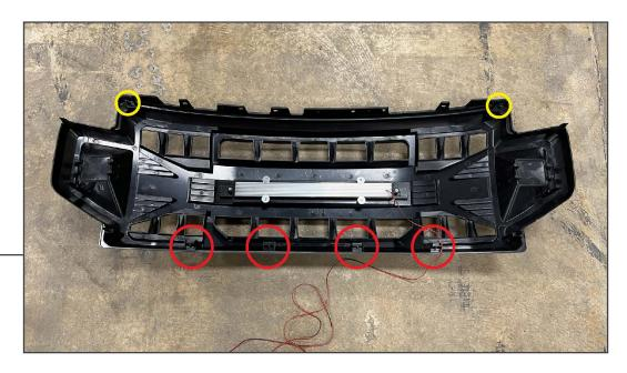
Transfer the (2) upper studs from the original grille to the new grille. Fit the included (4) clips to the bottom of the grille.
