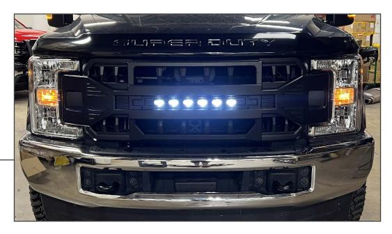
Re-install the radiator cover to the vehicle reusing the original plastic clips.
