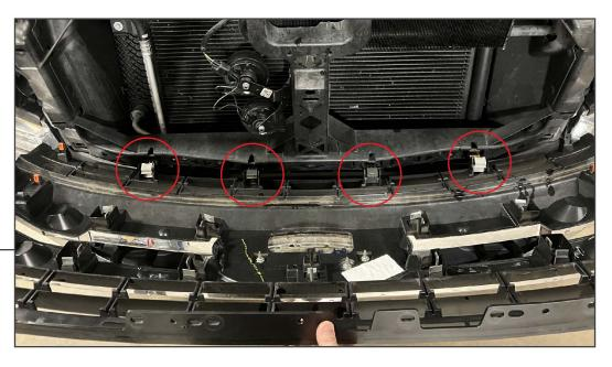
Begin pulling the top and sides of the grille away from the vehicle. Using a long flathead screw-driver, press the (4) lower metal retaining clips while pulling the grille away from the vehicle to dislodge the bottom of the grille.
