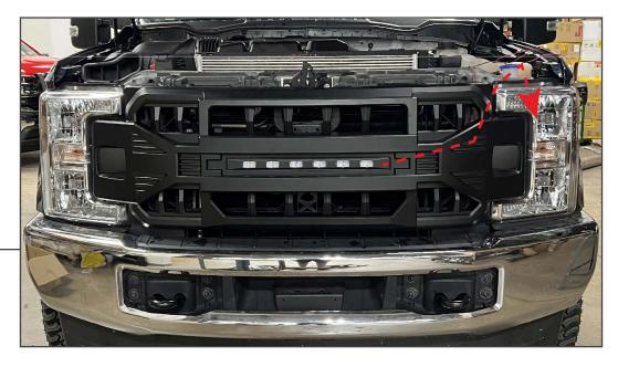
While holding the grille to the vehicle, route the LED lighting harness towards the driver's side headlight.
