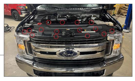
Open the vehicle hood. Remove (15) plastic push clips from the radiator cover. Remove the radiator cover from the vehicle.
