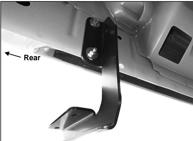
(Fig 7) Driver/left rear Mounting Bracket installed
