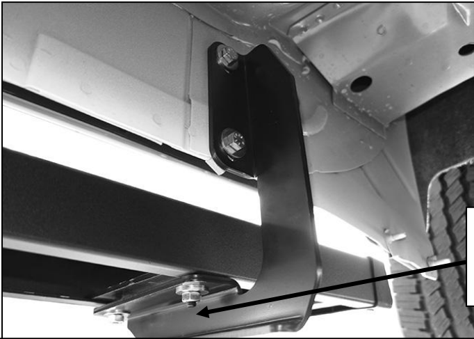
(Fig 10) Driver/left front mounting Bracket installed
