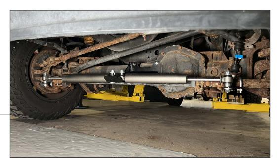
With the vehicle on the ground, turn the wheel lock to lock to verify the stabilizer shocks are the correct length. Adjust the stabilizer mounting points, if necessary to allow full shock travel/compression.
