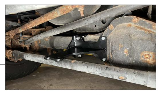
Secure the included axle mounting bracket to the front axle using (2) 3/8-16 x 1" bolts into the vehicle differential cover. Then, secure the opposide side of the bracket to the axle tube using (1) large U-bolt and (2) 3/8 flange nuts. Tighten all hardware evenly until fully secure.
