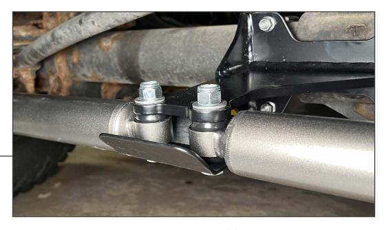
Fit each stabilizer shock to the center mounting bracket. Use the (1) axle clamp bracket under the stabilizer shocks, and secure into place using (1)  $1/2-13 \times 2.75$ " bolt, (2) 1/2" flat washers, and (1) 1/2" lock nut per stabilizer shock.
