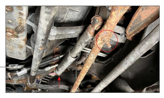
Locate and remove the original steering stabilizer from the drag link by removing (1) 18mm bolt and (1) 18mm nut.
