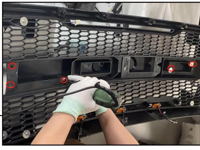
Open the hood,remove four 10-millimeter bolts along the top of the grille. Carefully lean the grille forward and locate the metal clips at the bottom, use a long flat blade screwdriver to push down and release these five clips. Then pull the grille off the truck.
