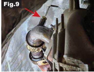
To remove the exhaust back pressure sensor tube, start by loosening the nut that holds the bracket in place. After that, loosen the flare nut that secures the tube. Next, detach the tube from the up-pipe and set it aside. **Fig.10**
