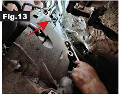
**Step 13.** Begin by installing the driver side PPE up-pipe, ensuring to use the supplied gasket along with the original 13mm nuts and v-band clamp. Similarly, install the passenger side PPE up-pipe, utilizing the supplied gasket along with the original 13mm nuts and v-band clamp **Fig.14**
