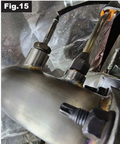
**NOTE:** For the installation of the driver side up-pipe, if additional clearance is needed, unbolt the transmission dipstick tube (do not remove)
