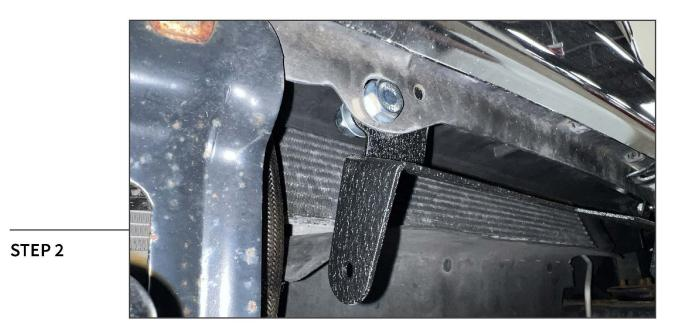
Fit the large mounting bracket holes on the bracket behind the bumper mounting holes, and loosely secure using (1) M12 x 30mm bolt, (2) M12 flat washers, and (1) M12 lock nut per side.
