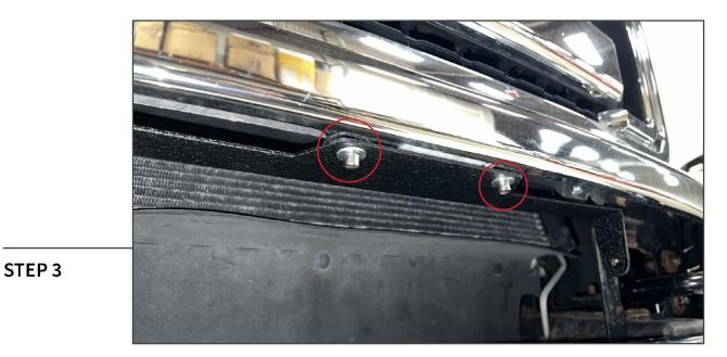
Secure the front of light bar bracket the center of the bumper using (2) M8 x 25mm bolts, (4) M8 flat washers, and (2) M8 lock nuts.
