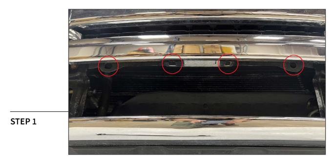
Along the center of the bumper, locate the (4) holes along the inside of the bumper.
