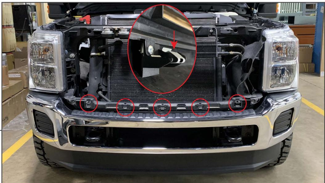
Slightly pull the top of the grille away from the vehicle to locate the lower metal mounting clips. Using a flathead screwdriver, disconnect the (5) metal clips securing the bottom of the grille to the radiator support. Remove the grille from the vehicle, and place on a soft surface for disassembly.
