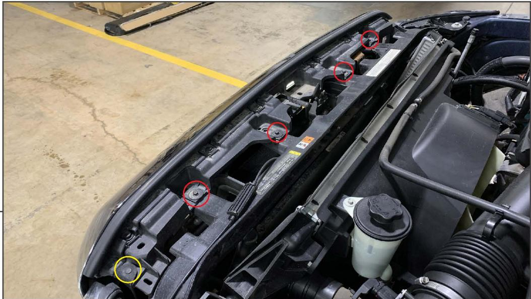
Open the vehicle hood. Using a panel removal tool, remove the air dam plastic push pin. Remove (4) 10mm bolts along the top of the grille.
