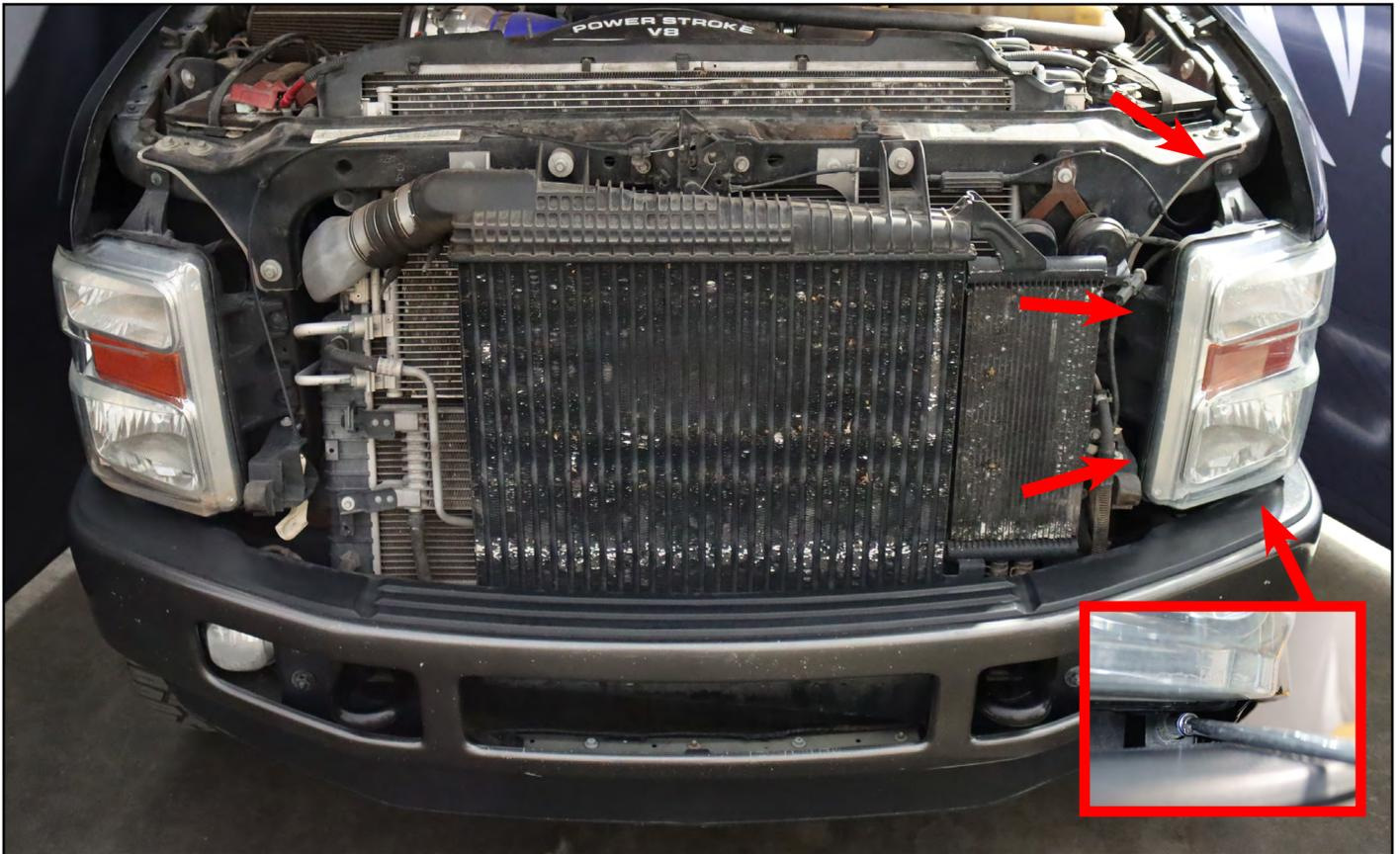
After removing the bolts, carefully pull the headlight forward and unplug the light sockets to facilitate headlight removal. Repeat the same steps for the other side.
