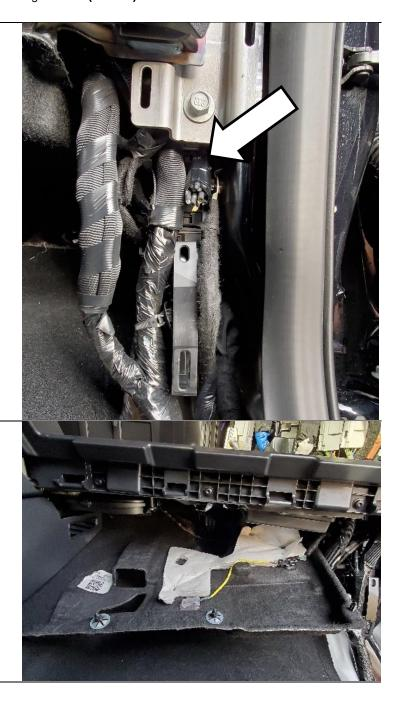
The pigtail location has been found to vary from truck to truck. Shown here is the most hidden and inaccessible spot. The metal bracket that held the plastic panels can be used as a reference point.
