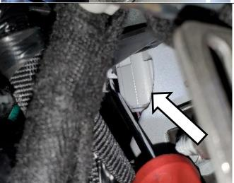
Pull the pigtail free so that the grey connector is visible and can be disconnected. The connector may be clipped in and may require a firm pull to pull down.
