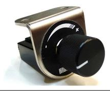
Installation without bracket. Drill a 9/32" hole in the dash to mount the switch. Beside the first hole, drill a 1/8" hole for the locator tab. Use the switch as a guide for location. Apply the switch decal to the dash and insert the switch through the dashboard. Install retainer nut. Install the knob on the switch using a 1/16" Allen key. Plug the harness into the back of the switch.
