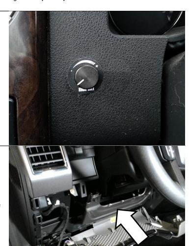
If mounting in the knee bolster, be aware of the reinforcement plate behind the bolster, which will limit the available spaces to mount the switch.
