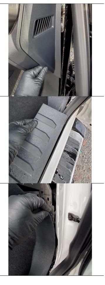
On some 2023+ trucks, the up-fitter pigtail is accessible after removing the kick panel. The pigtail can be identified by the bundle of wire terminals taped together and connected to a grey connector.
