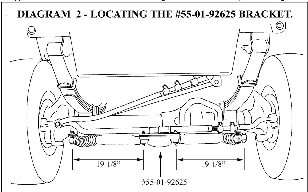
position the bracket so that the distance between the stabilizer mounting studs on the axle and the studs on the "02" bracket is 19-1/8". Tighten (26).
