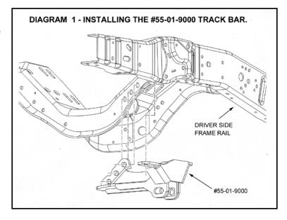
the upper mount and the cam bolt in the lower. All hardware should be installed from the outside. Snug, but do not fully tighten at this time.
