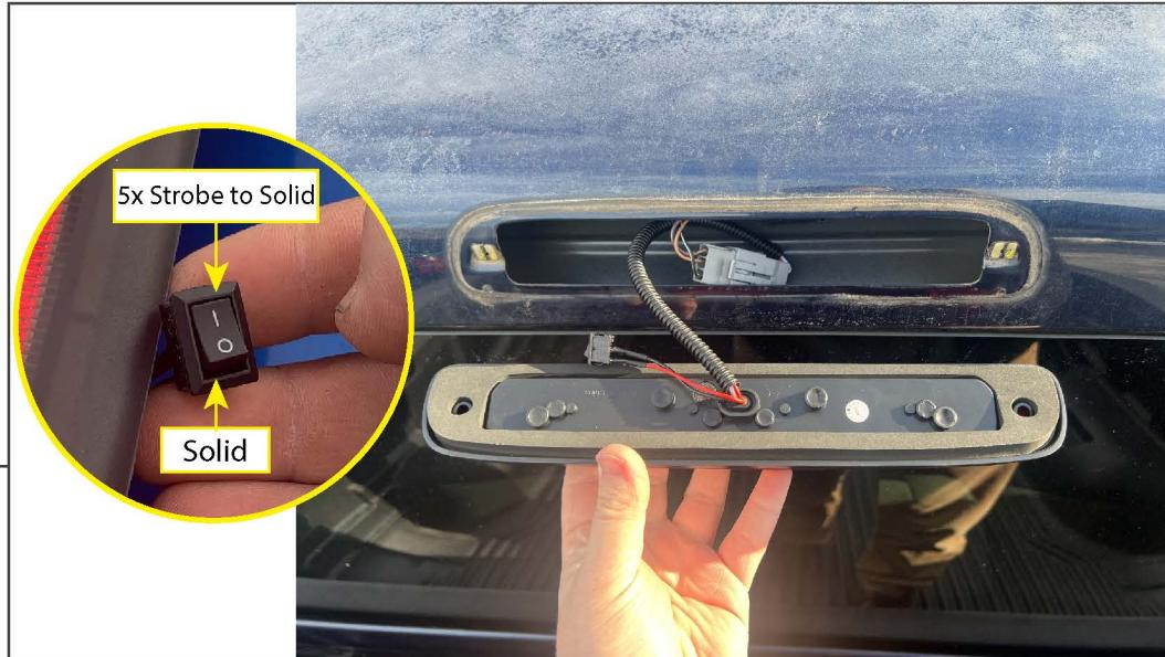
Plug in the brake light electrical connector into the vehicle's wiring harness. Toggle the switch to enable 5x strobe feature.
