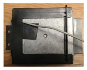
Be sure the box holding the computer in place does not bind the chip causing it to tilt and lose connection. Return the ECM to its location and re-connect the wiring harness and 2 bolts in box. Reconnect Batteries.
