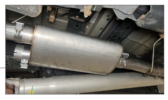
Fit the muffler onto the front pipe. Support the muffler into place with a floor jack. Loosely secure the muffler to the front pipe using the previously placed clamp.
