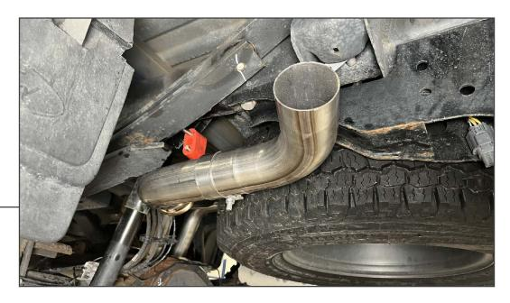
Fit the exit pipe onto each side exhaust pipe, and loosely secure using the previously placed clamp on each side.
