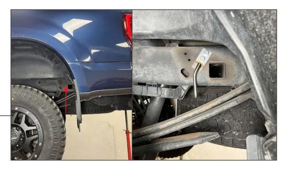
Along the driver's side frame, locate the threaded bolt holes in the frame. Secure the included hanger bracket to the frame utilizing the bolt holes with the included (2) M10x1.50 x 20mm bolts, (2) M10 lock washers, and (2) M10 flat washers.
