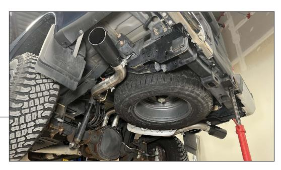
Lower the vehicle to the ground to allow the suspension to become loaded. Adjust the exhaust into the desired position, and tighten all exhaust clamps to secure the exhaust into place. Torque all clamps to 45 ft. lbs.
