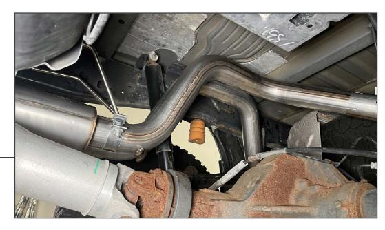
Fit the LH over-axle pipe into the muffler, and then fit the pipe hanger into the vehicle rubber hanger above the muffler. Loosely secure the LH over-axle pipe to the muffler using the previously placed clamp.
