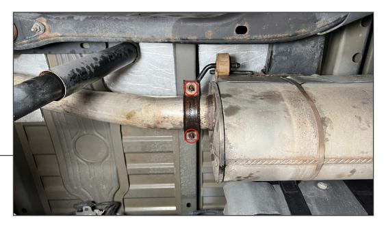
Remove (2) 13mm nuts from the rear of the muffler assembly. Then, remove the hanger bracket from the vehicle frame.
